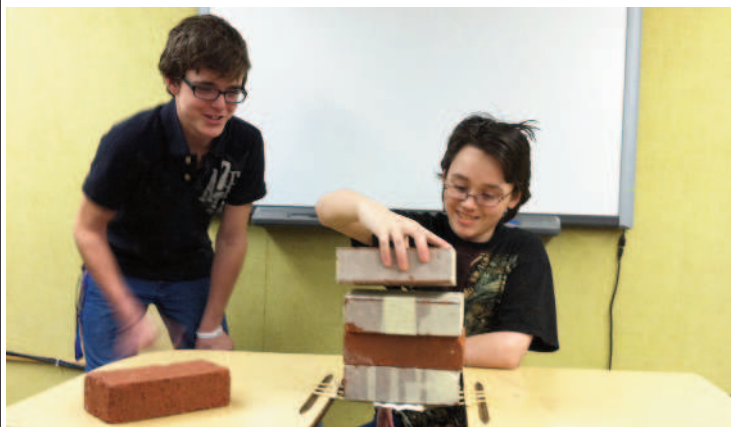
Tim Maynard and Cade Prime carefully balance bricks on their bridge made of athletic tape and popsicle sticks.
